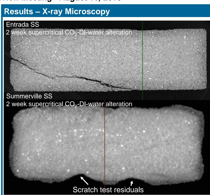
μCT images of Entrada Sst (top) and Summerville Sltst (bottom) samples after 2 weeks alteration at 1350 psi  $CO_2$  and 80°C with deionized water. Darker periphery regions show porosity increase. Alteration induced dissolution was the likely cause for the crack in the Entrada sample.
