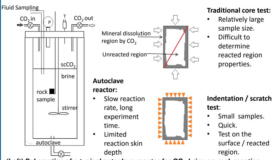
(Left) Schematics of a typical autoclave reactor for CO<sub>2</sub>-brine on rock reaction. (Right) Comparison between traditional core-scale test and indentation & scratch tests on CO<sub>2</sub>-reacted rock samples. (Below) Labeled picture of experimental setup
