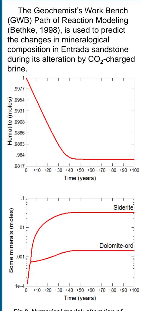
Fig.8. Numerical model: alteration of Entrada sandstone by CO<sub>2</sub>-charged brine. Hematite dissolution (top), and siderite and dolomite precipitation (bottom) are predicted.
